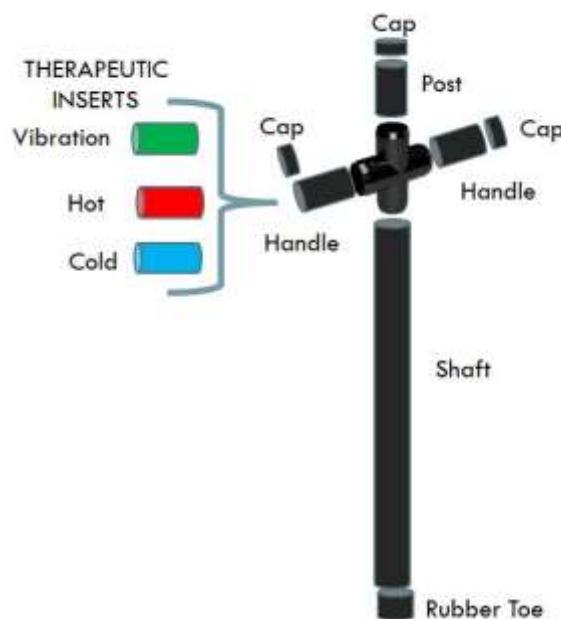
Figure 5 - Hybrid model with color coded inserts
